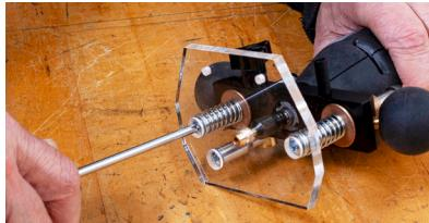
Now you can remove the indexing pin and chuck a 1/16" downcut bit in the rotary tool. Note: While an upcut bit could work, you run the risk of compacting dust under the inlay plate. A downcut bit will push the dust into the pocket, keeping the bit clear.
