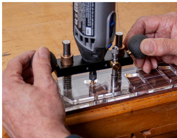
Setting the plunge depth with the jig and templates can be done on any flat surface or fingerboard.
