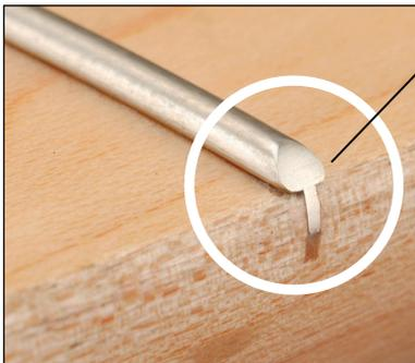
**Shape and polish** Slightly round off and smooth the ends of each fret using the Fret End Dressing File. This file has two smooth edges that can ride on the fingerboard without cutting: use the rounded edge for a rolling action when you round the fret ends.
