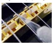
lightly scribe marks on each side of the string. File a slot between the scribed lines, constantly checking that you're keeping proper string placement. Cut slots this way for all the wound strings.
