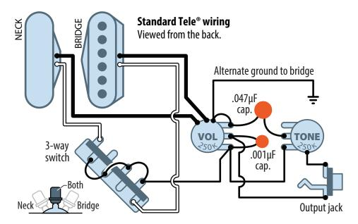
**Our Tele neck pickup is RWRP.** Stewmac pickups are designed to capture the tone and response of late '50s originals. Unlike vintage pickups, our Tele neck pickup is reverse-wound with reversed polarity magnets (RWRP). This gives you hum-cancelling output in the middle position of the 3-way switch.
