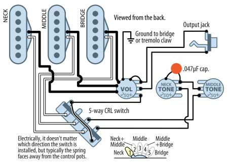
Standard three single-coils with one volume and two tone controls
