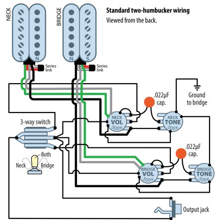
**Independent pickup volumes:** To blend the pickups independently, swap the wires from the pickups and the switch where they connect to the volume pot. This solves the problem in the middle position of the switch where turning down one volume control affects both pickups.
