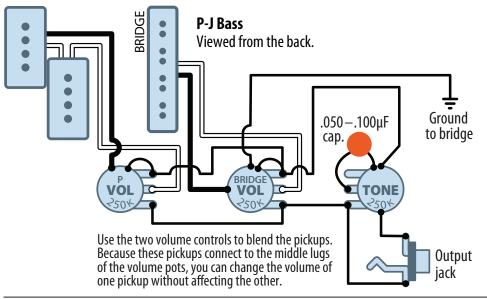
**Setting your pickup height:** For neck pickups, try about 1/8" between the polepieces and the bottom of the strings when fretted at the highest fret. For bridge pickups, try 3/32". Experiment to find what sounds good to you: closer to the strings will sound louder and grittier, farther will sound clearer and guieter.
