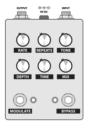
**Time:** From about 30ms fully counterclockwise to about 625ms fully clockwise.
