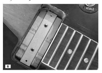
When installing the mounting bracket in a routed cavity, it's important to center it correctly. To do this, make scrap wood spacers. In this photo, a disassembled clothespin worked perfectly.
