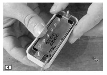
Slide your assembled pickup over the height adjustment screws. Because you drilled out baseplate ears in the first step, the pickup slips over the screws and down onto the two plastic spacers.
