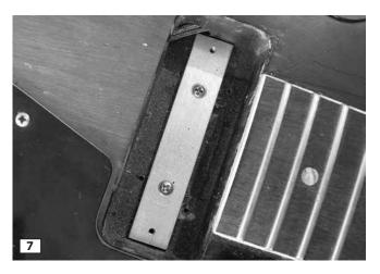
Drill two 5/64" holes for the mounting screws and install the bracket. The mounting bracket is now ready for you to install the mini-humbucker pickup.
