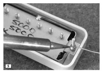
Thread the hex nuts onto the height adjustment screws and tighten them so the pickup fits tightly against the plastic spacers. Solder the nuts onto the height adjustment screws so they cannot be removed.
