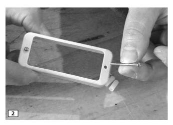
Slide the height adjustment screws into the mounting ring.
