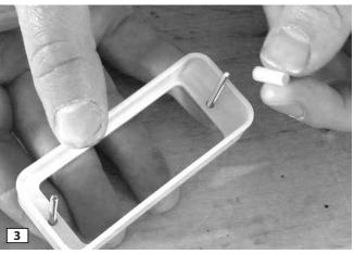
Holding the height adjustment screws in with your fingers, flip the mounting ring over and slip the plastic spacers over the screws.
