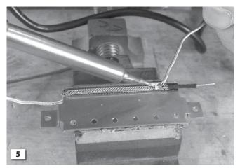
Holding the baseplate with a vise or clamp, solder on the hookup wire.
