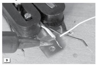
Solder the two white leads together for your series link. Tape off the joint and tuck it between the two bobbins.
