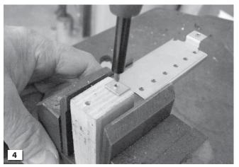
The two "ears" on the metal baseplate have threaded holes for height adjustment screws. For a Deluxe mount, these holes need to be enlarged so they'll slip over the screws without the threads engaging.
