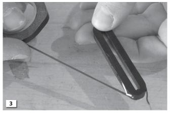
Give the bobbins a few wraps in paper coil tape to secure the lead wires. This is delicate work; be very careful not to break the leads as you wrap.
