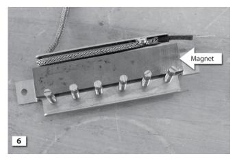
Determine the south side of the magnet using a polarity tester, and place the magnet on the polepieces, south side up.
