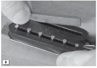
Place the two bobbins on the baseplate. One over the screws and the other next to it sitting on the magnet. Install the steel slug in the bobbin.
