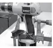
We fashioned a mounting plate in the shape of the pickup (with a recess for the eyelets), and mounted that onto a metal shaft that's held in the drill chuck. Whatever your method, see that the pickup is spinning true and straight.
