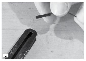
Solder the black lead to the start tail and tape the joint using coil tape. Do the same with the white lead and the finish tail. There's no need to strip the clear insulating coating from the fine coil wire; the heat from soldering will melt it away.
