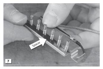
Insert the plastic spacer between the polepieces and side of the bobbin.
