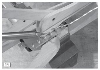
Use a second clamp to gently squeeze the sides of the cover to fit tightly against the baseplate. With a hot soldering iron, put one small dab of solder on each side of the cover to secure it.
