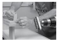
adjustable right and left limiters. For this simple winder, the limiter is a hole drilled in a piece of wood that pivots right and left. The hole needs to be sanded very smooth.
