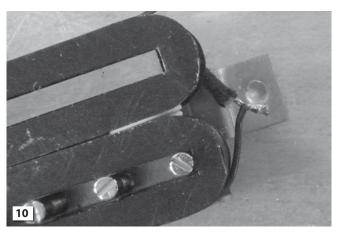
Solder the black start lead of the polepiece coil to the hot, center lead of the hookup wire.
