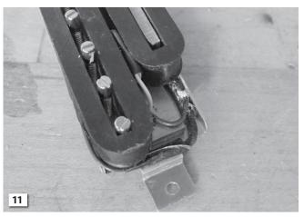
Finish by soldering the start of the slug coil to the braided shield of the hookup wire. Carefully tuck all wires out of the way to make room for the pickup cover.
