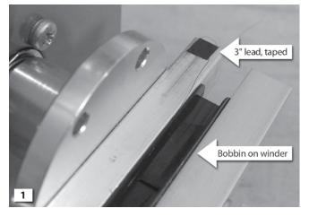
Wind 42 AWG coil wire around the bobbin by hand, giving it about six turns counterclockwise, leaving a 3" tail. This tail will be the pickup's start lead; carefully tape it to the platen of the winder, keeping it taught so it's out of the way of your winding.
