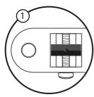
STEP 1. Once you have removed the old saddles and replaced them with your new fraph Tech saddles, set the intonation "starting point": screw the intonation screw so that the saddles are close to the centre of the bridge. Tune your guitar to concert pitch.
