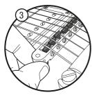
STEP 3 . To adjust your string height, adjust the two thumb wheel screws up or down until correct string height is acheived. Tune guitar to concert pitch after each adjustment.
