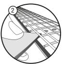
STEP 2 . To determine correct string height, measure the gap between the top of the twelfth fret and the bottom of the low E string. It should be around 3mm/.118", or about a stack of 12 business cards if you don't have a ruler. For the high E string, the gap should be around 2mm/.079", or about a stack of 8 business cards.
