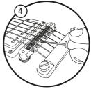
STEP 4. The fretted 12th position of a string should match its 12th fret harmonic (lightly touch the string right above the 12th fret and pluck). Adjust the intonation screw with a screwdriver. Shortening the distance between the saddle and nut will increase the pitch of the harmonic; increasing the distance lower the pitch. Retune to concert pitch after each adjustment. Repeat for each string.
