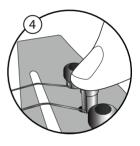
Pull up on the string to slide the ball end up the bridge pin and anchor it against the bridge plate, then push the pin down into the tapered hole. The pin does not have to be tight to hold the string firmly. Push gently to seat the pin.
