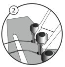
Remove your old bridge pins using your fingers or a pin puller like the one on the end of most string winders.
