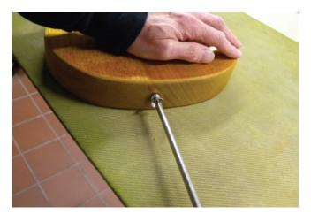
During assembly, use a padded surface to protect the finish from scratches and dents.
