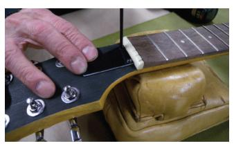
Mark out the truss rod cover Drill the holes using a 1/16" bit, drilling 3/16" deep.
