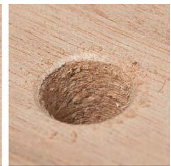
Bushing hole with chamfer
