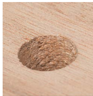
Bushing hole before chamfering
