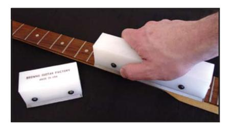
After the frets have been installed, place your **Fret Beveling File** on the fingerboard. Run the file along the full length of the neck, simultaneously beveling all the fret ends until they're flush with the fingerboard. Then round the fret ends with a 3-corner fret dressing file. If necessary, remove any remaining imperfections by lightly sanding and buffing, and use a proper wood oil. Always protect any areas of the instrument that are not being worked on.
