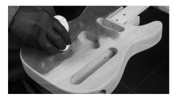
After each coat, allow to dry 2–3 hours. It may be necessary to scuff-sand between coats to ensure a level build of coats. To scuff-sand, fold 400-grit sandpaper around a foam block, and make light passes to knock off any high spots. Make sure all dust is removed before applying your next coat.
