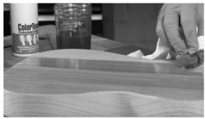
400-grit sandpaper and a block (making sure to not sand into the color coats). Remove all dust and apply a final coat of clear finish.
