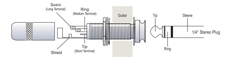
Our new **SWITCHJACK**<sup>TM</sup> T•R•S•S (Tip/Ring/Sleeve/Switch) Stereo Switching Endpin Jack allows simultaneous stereo operation and battery switching. This new configuration now simplifies stereo wiring with many pickup combinations that were previously incompatible.
