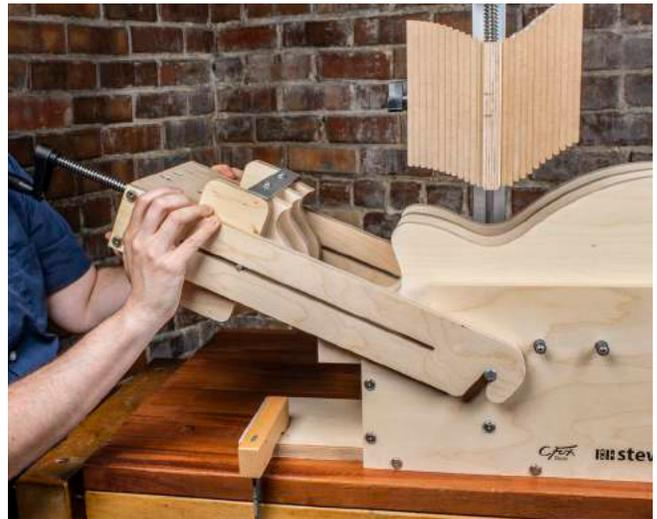
Use the crank on the Cutaway Ram to lower the cutaway mates completely into the cutaway of the Bending Forms.
