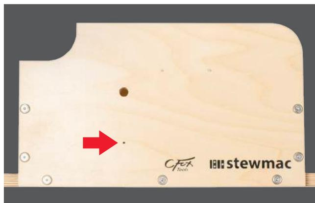
Lay the now-connected base and waist clamp on the back of the waist clamp. Install the three Torx drive screws in the pre-drilled holes in the base and wooden insert of the waist clamp and tighten. Install these in tandem for even pressure. Sit the bender back upright.
