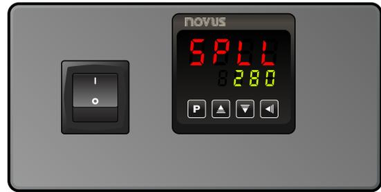
To set the maximum temperature, press the **P** button again and you will see "SPHL" (Set Point High Limit). Use the up and down arrow buttons to set the desired maximum.
