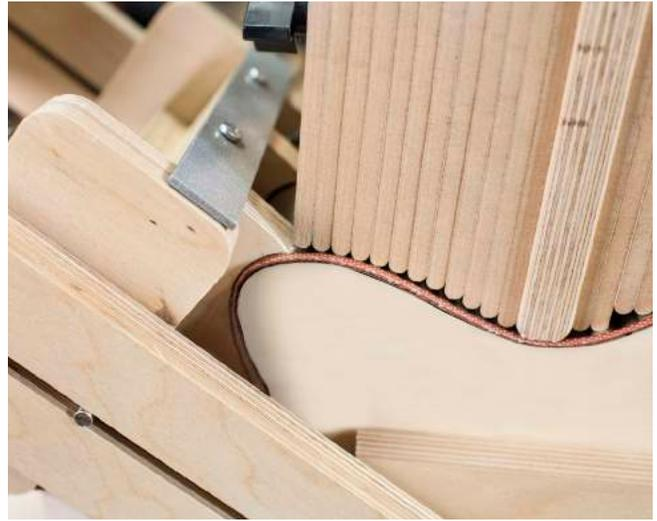
Once the Cutaway Ram is fully mated, turn off the Temperature Controller. Let the wood set and cool for 10-15 minutes before removing the side.
