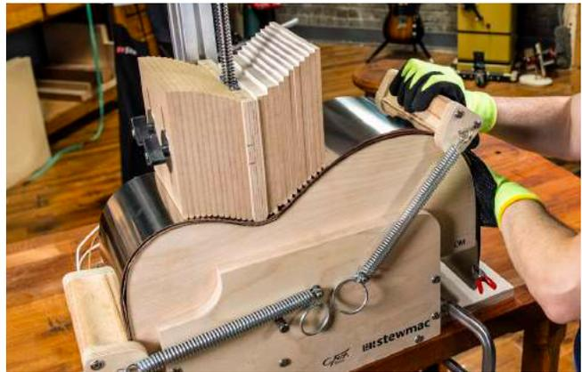
Once you get near the contour plates, use two hands to prevent the pressure bars from slamming into the plates.
