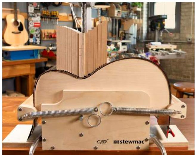
Once the waist clamp is tightened, turn off the power to the controller. Let the wood set and cool for 10-15 minutes before removing the side.
