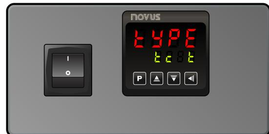
Press and release the **P** button to toggle through the menu until you see "unit" displayed in red. The green text will read °F for Fahrenheit or °C for Celsius. Press the up or down arrow buttons to change to your desired unit. Once changed press and release **P** to continue through the menu.
