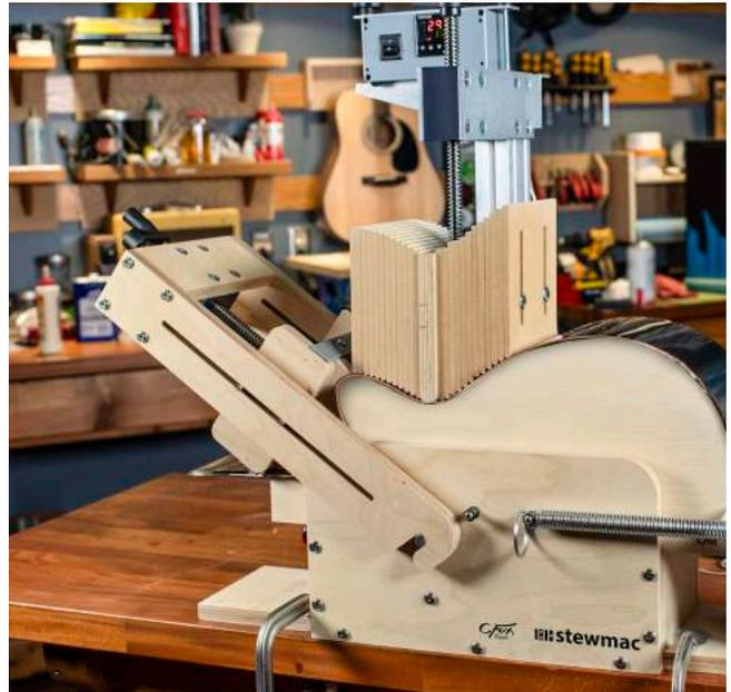
Crank the waist clamp up and remove the sandwich and bent side.
