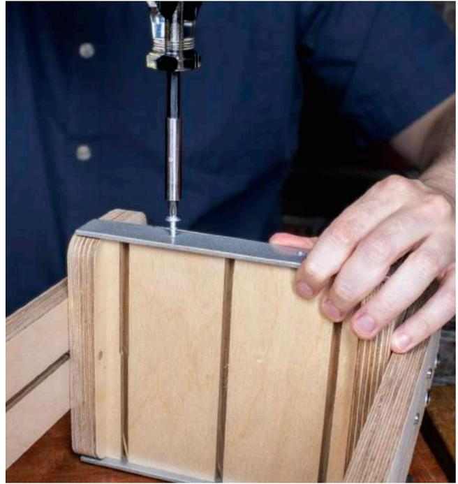
Unscrew the front retainer plate on the Cutaway Ram to expose the screw slots. Slide the cutaway mates into the slots, making sure they match the cutaway in the Bending Form. If the cutaway mates are difficult to slide in, adjust the screws on their undersides so they slide in snugly.
