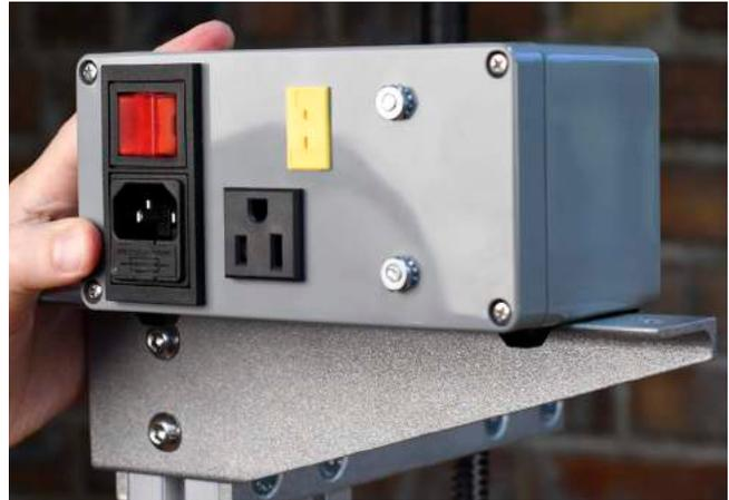
Place the top bracket plate on top of the controller. Insert the threaded rods through the holes in the top bracket plate, with the knobs on top. Place the threaded rods through the matching holes in the bracket and secure with the wingnuts.
