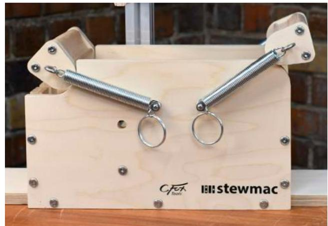
Test fit each pressure bar by attaching the spring hooks to the front spring mounts on the front of the base. Make sure the spring hook, NOT the ring handle is secured to the mount. The ring handles are for moving the springs only.
