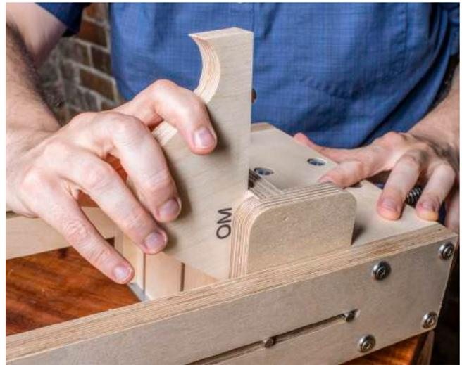
Reinstall the retainer plate. Note the holes in the plate are offset. Make sure that the plate is oriented to fully contact the mates when reinstalled.
