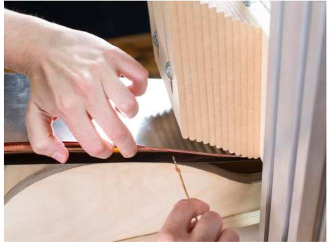
Install the lower bout pressure bar over the sandwich. It should ride over the edges of the sandwich and Bending Forms and rest against the waist contour plates. Take care to install the spring hooks onto the spring mounts, and not the ring handles.
