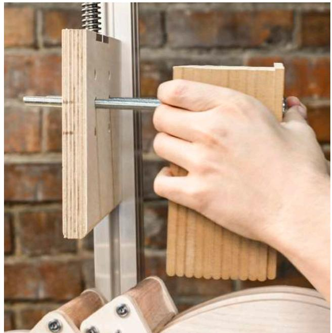
Stack the remaining twelve contour plates (rounded sides down) and slide them onto the carriage bolts sticking through the center plate.
