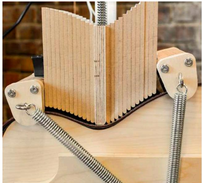
Slowly pull the lower bout pressure bar down to start bending the lower bout. Take your time and pull it down until it's right at the end of the form. You may need to remove the mini clamps to completely lower the pressure bar. This bend should take 2-3 minutes.
