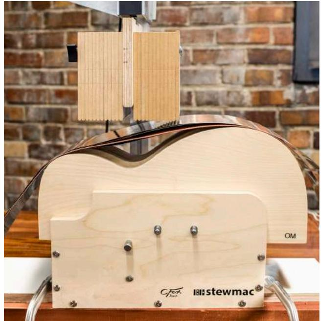
Slightly loosen the two knobs holding the contour plates together so they can move freely. Crank the waist clamp down until the straps and blanket conform to the waist shape.
