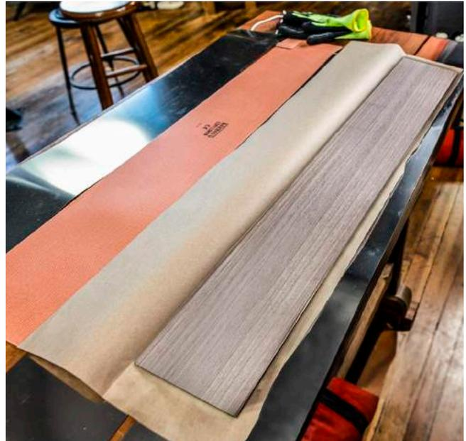
Lightly spritz both surfaces of the guitar side and the interior of the wrapping with distilled water or Super-Soft 2 Veneer Softener. Lay the guitar side back into the wrapping with your waist mark and "B" facing down (toward the floor) and the tapered neck end of the guitar side pointing left toward the upper bout.
