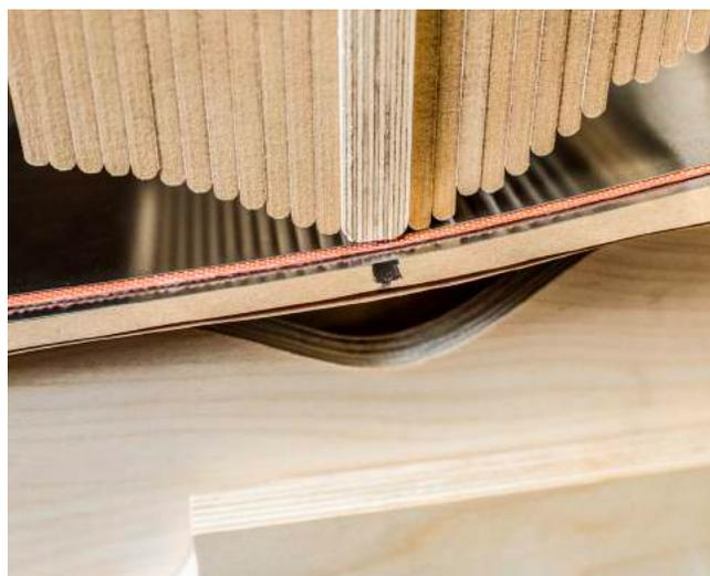
Make sure the upper bout pressure bar is positioned between the back of the bender and the waist clamp as shown. Once the waist clamp is lowered you will not be able to reposition it.
