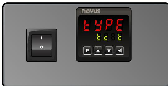
To set the minimum temperature, press and release the **P** button until you see "SPLL" (Set Point Low Limit). Then use the up and down arrow buttons to set the desired minimum temperature.
