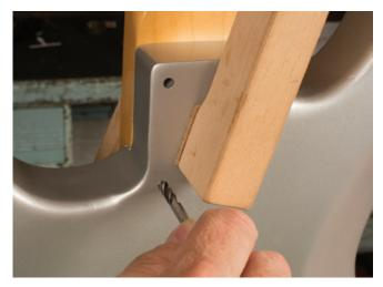
Use the holes in the body to mark the neck. A scribe, nail, or transfer punch will make clean marks in the neck to show you where to drill. A 4mm brad point drill bit turned by hand also works well for making these marks.
