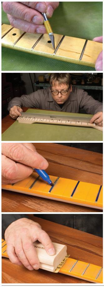
After the finish has cured, it's time to level and dress the frets. If you have a maple fretboard, lightly score the lacquer along the length of the frets with a sharp knife, using care not to cut into the wood or scratch the frets. This step helps in removing the lacquer that was sprayed over the frets during finishing.
