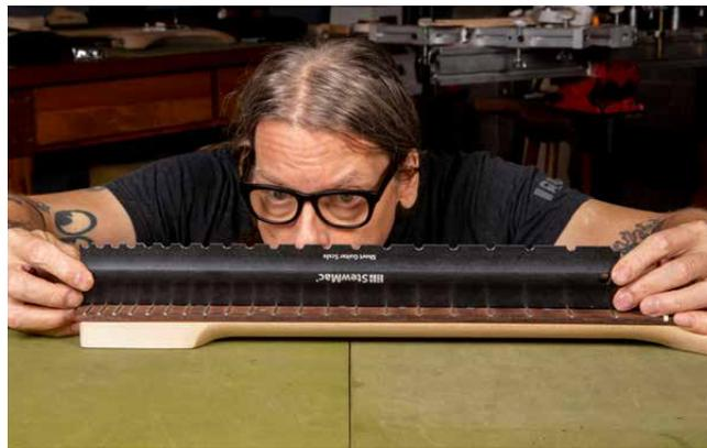
Turn the truss rod nut counterclockwise to bring the neck up, adding relief.
