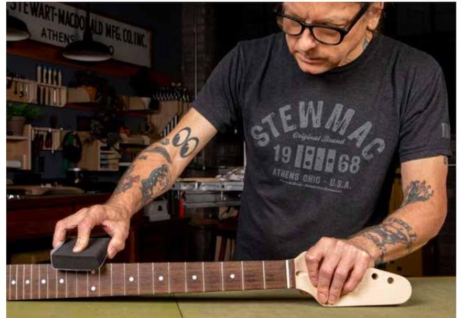
After a complete sanding, wipe down the body and neck with a damp cloth to raise the grain to reveal fibers that need more sanding. Let the wood dry, then sand the raised grain with 220-grit sandpaper. After sanding, raise the grain again and sand a third time, using 320-grit sandpaper.
