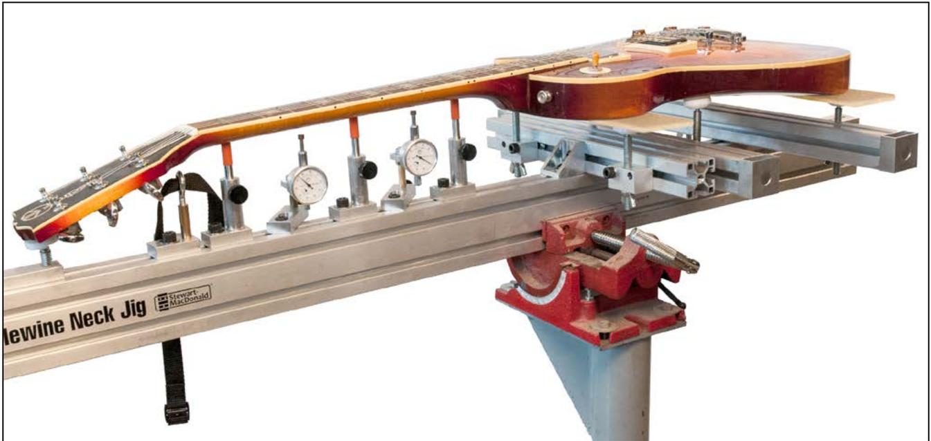
**3.** Gently set the guitar on the body levelers (and paper-wrapped slats, if you're using them). A sandbag or padded weight placed on the guitar body is a helpful temporary weight to keep the guitar from moving as you position the body on levelers and center the neck over the support rods. Adjust the height of the levelers so that the fingerboard is approximately parallel with the main beam. The lower you can set the levelers the better — for solid, stable support.
