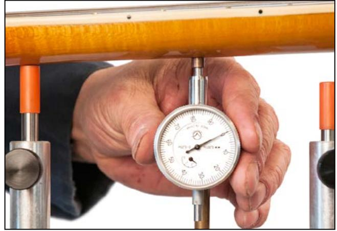
**7.** Set each dial to zero by turning the indicator's outer ring. Turn the dial to zero, then turn it past zero by two full rotations before arriving at zero again. These extra rotations give the dial room to move and adjust on either side of zero as you adjust the neck. The thumbscrew locks the outer ring.
