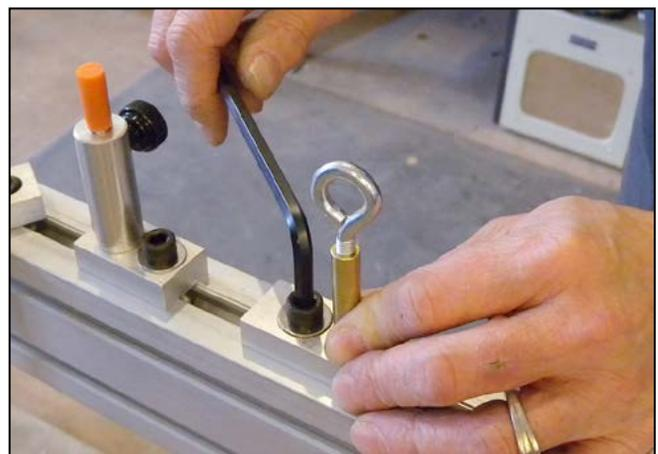
**7.** Attach the peghead puller and thread the strap through the eyebolt.
