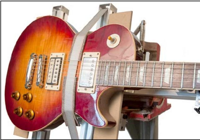
**6.** With the guitar tuned to pitch, move the Neck Jig onto its side (the playing position). Adjust the neck for fret leveling or dressing; the truss rod should create backbow when tightened and create relief when loosened. You want the neck to be straight for fret work.
