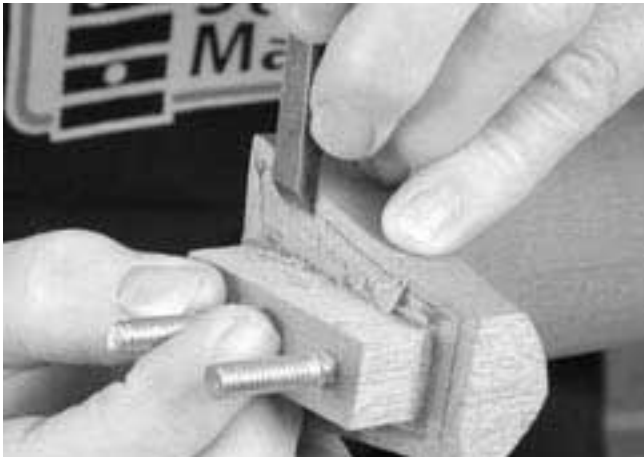
16. Use a sharp chisel to remove wood from the inner area of the neck heel cheeks.
