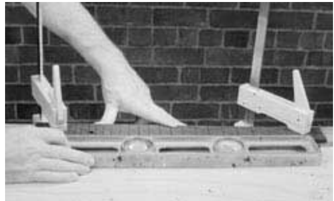
5. Clamped and sanded in this fashion, the fretboard will not only be straight end-to-end, but the edge will be sanded at 90°.
