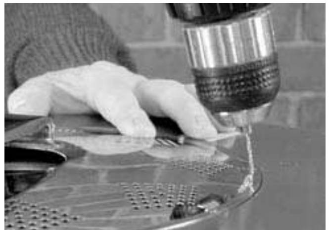
33. Tilt the drill bit slightly to remain square to the lip and to ensure that you drill into solid metal.
