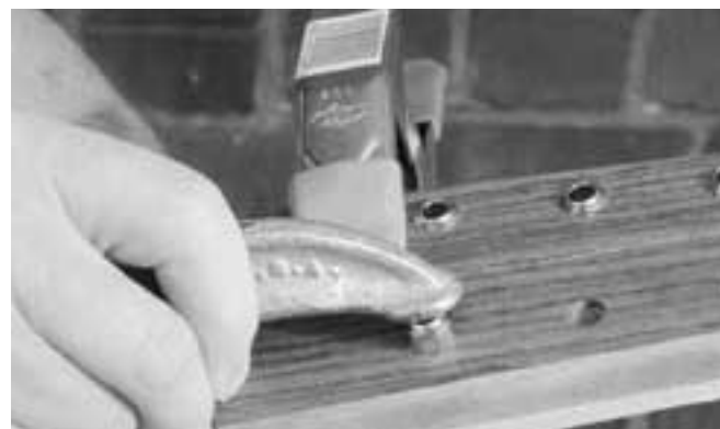
32. Press the bushings into the holes in the peghead overlay using a clamp to apply firm, even pressure.
