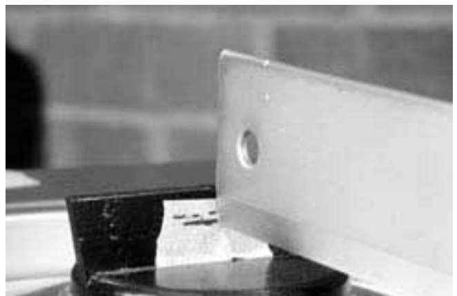
36. On our guitar, the bottom of our straightedge was 3/8" off the face of the biscuit.
