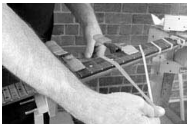
26. Hold the fingerboard in place with a spring clamp as you start to wrap with the rubber bands.
