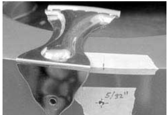
12. Place a piece of masking tape on the sides at the tail block end of the body and transfer the centerline onto the metal sides there.
