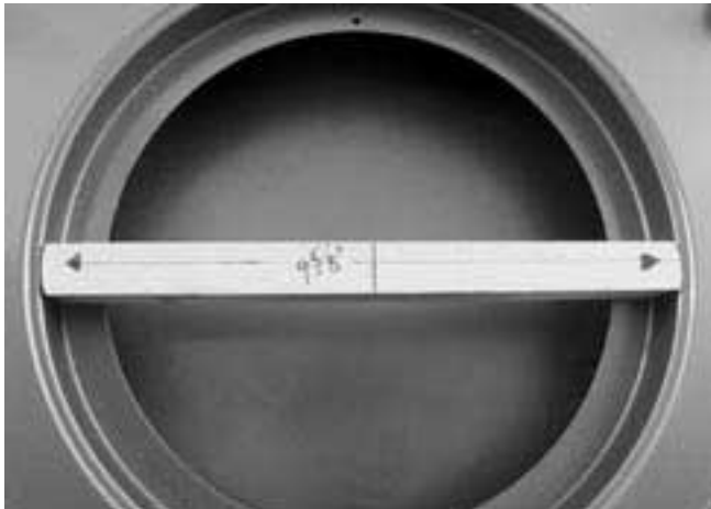
10. From scrap wood make a "centering stick" 9\text{-}5/8" x 1\text{-}1/16" .
