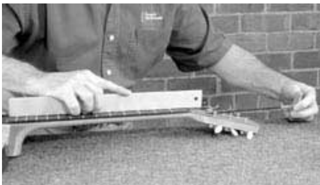
38. Adjust the neck perfectly straight, until a straightedge rests on all the frets.
