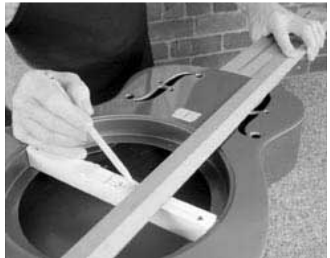
21. Use a straightedge laid against both the treble and bass sides of the fretboard to check neck alignment to the body centerline.
