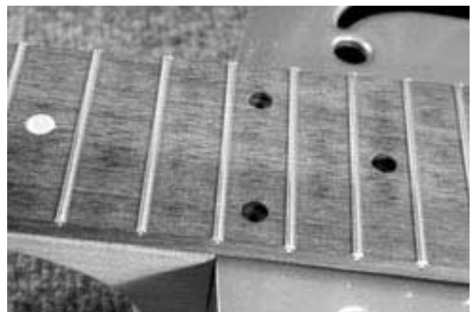
24. Locate the fingerboard so that the 14th fret lines up with the outer top edges of the cheeks where they join the body.
