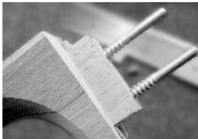
15. The tenon will now fit through the rectangular hole in the body.
