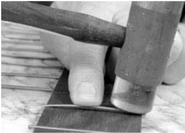
7. Keep the wire from tipping and prying up a chunk of wood as you tap the two ends into the fret slot with a hammer.
