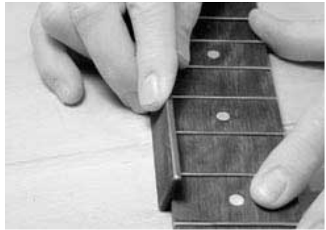
8. Use a smooth mill file, held at an angle, to bevel the fret ends.
