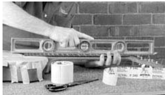
39. Use 240-grit or finer sandpaper double-stick taped to the narrow edge of a long flat surface.
