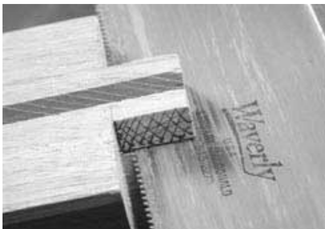
14. Saw in from the back of the tenon on each penciled line.
