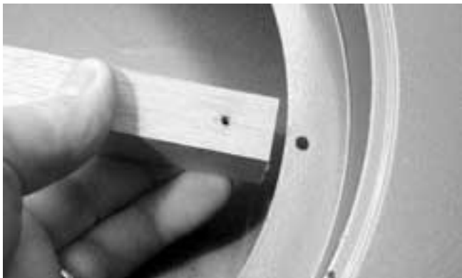
35. Remove the support and drill two mounting holes.
