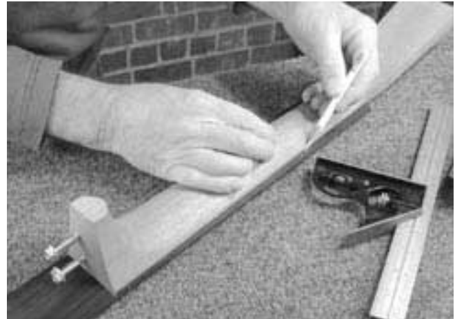
4. Draw the profile of the neck's taper onto the fingerboard using a white pencil.
