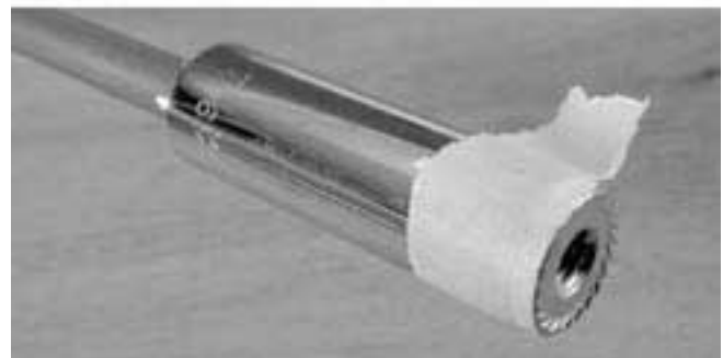
19. A #3 Phillips screwdriver fits the 1/4" square-drive. Use tape to hold the hex nut into the socket.
