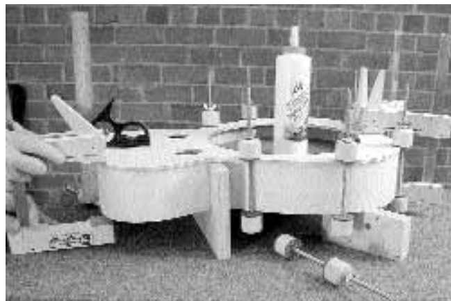
6. Start clamping in the waist area, for several inches to either side of the waist clamp, using spool clamps to gently hold the top in place.
