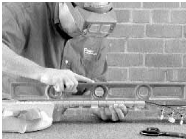
40. We used a carpenter’s level and 320-grit sandpaper to level the frets.
