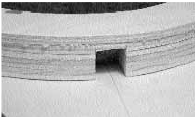
7. Don't cut entirely through the spacer to the soundwell bottom ring.
