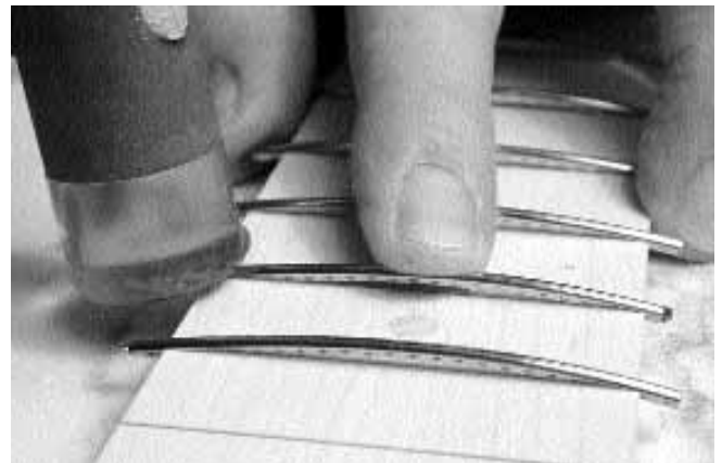
15. Keep the wire from tipping and prying up a chunk of wood as you tap the two ends into the fret slot with a hammer.
