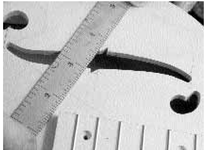
34. Use a thin triangle file and knife to cut angled notches.
