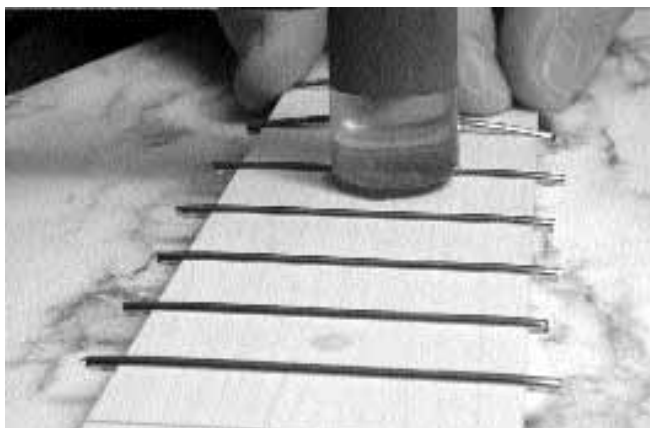
16. The fret tang, with its diamond-shaped barbs, embeds itself into the fingerboard as the fret straightens.
