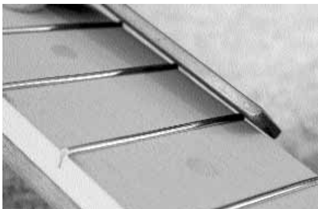
18. Use a smooth mill file, held at an angle, to bevel the fret ends.
