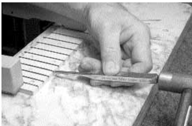
17. Just like Leo Fender did for 50 years, we opted to tap the frets over sideways slightly.
