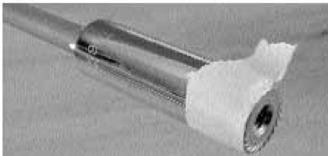
21. We made a long-handled nut driver from a deep-well, square-drive 7/16" socket, and a #3 Phillips screwdriver that fit the 1/4" drive perfectly.
