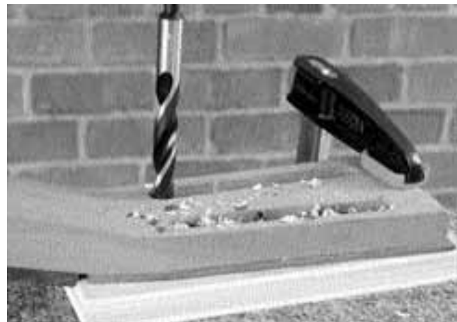
35. Use a 7/16" drill bit to drill holes against each end of the tuning machine channels.
