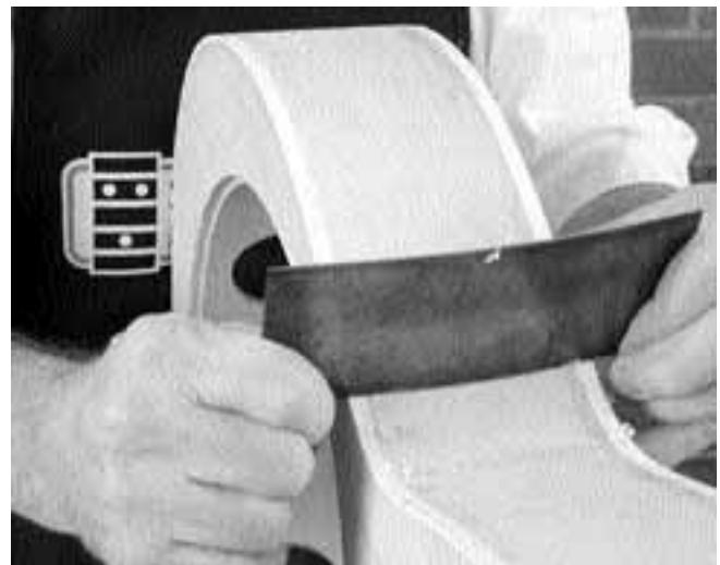
19. Scrape the wood to meet the binding all around the sides.
