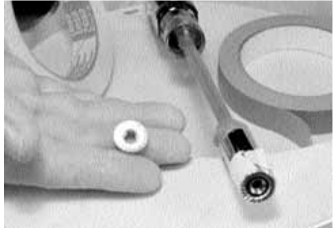
39. We made a long-handled nut driver from a deep-well, square-drive 7/16" socket, and a #3 Phillips screwdriver that fit the 1/4" drive perfectly.
