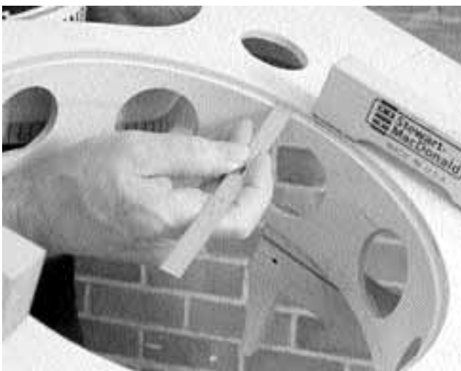
10. This ledge supports the cone and the spider; it's not very wide, so you must carefully center the sound well when gluing.
