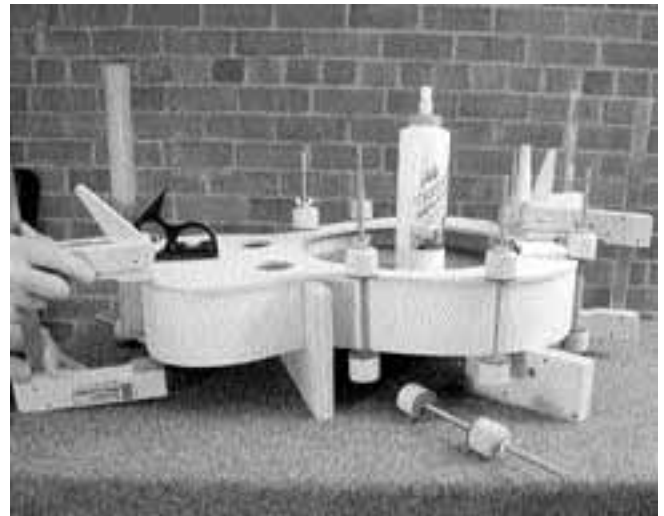
6. Start clamping in the waist area, for several inches to either side of the waist clamp, using spool clamps to gently hold the top in place.
