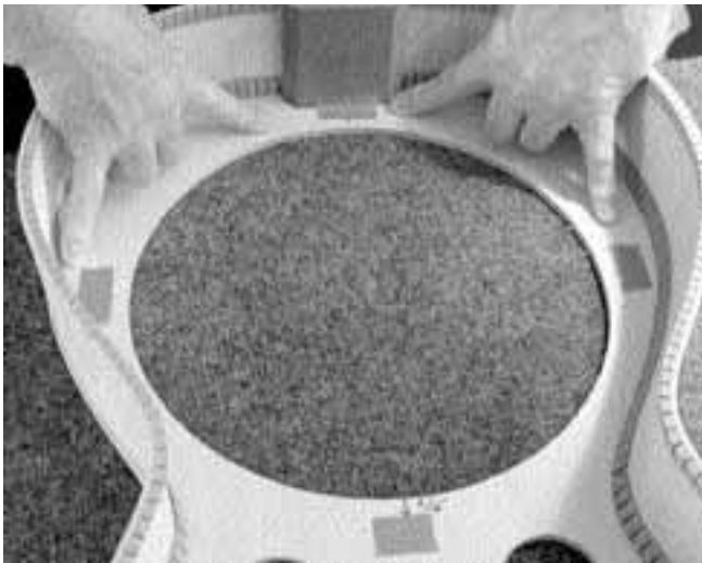
8. Masking tape placed at four opposite points helps you align the sound well.
