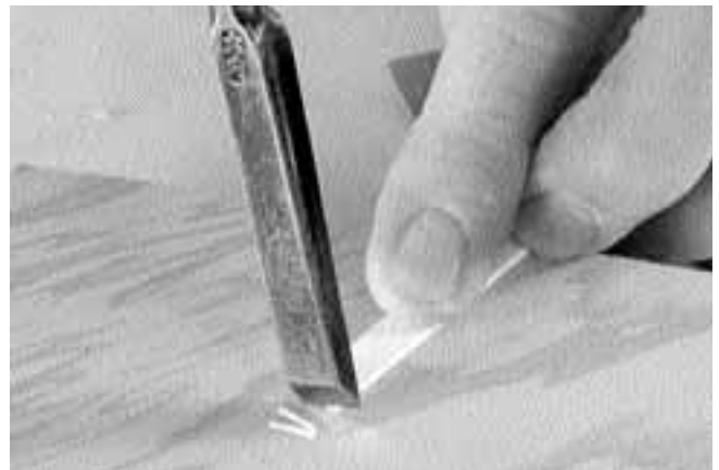
15. Trim the binding square at the starting point so that the butt-jointed seam between the two halves is tight.
