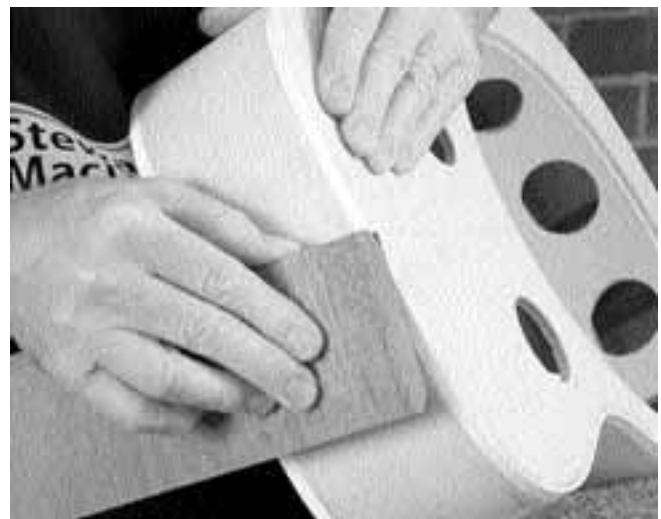
20. Use a flat block and 80- or 100-grit Fre-Cut® sandpaper to flatten only the area of the sides at the neck block where it mates with the flat cheeks of the neck.
