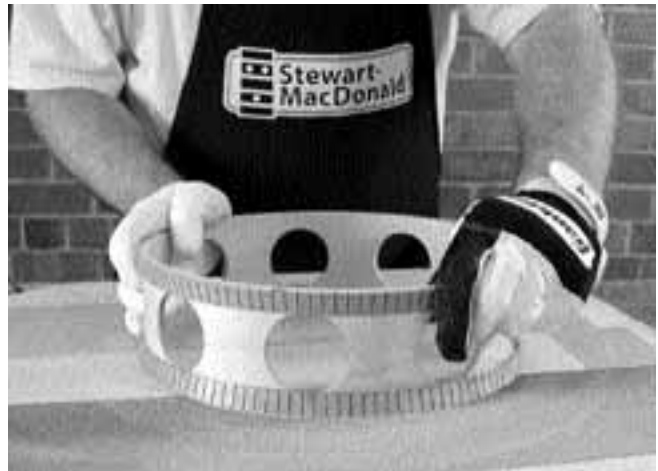
7. Flush-sand only one kerfed edge of the sound well — the edge that glues to the top — then flush-sand the back edge after the sound well is glued to the top.
