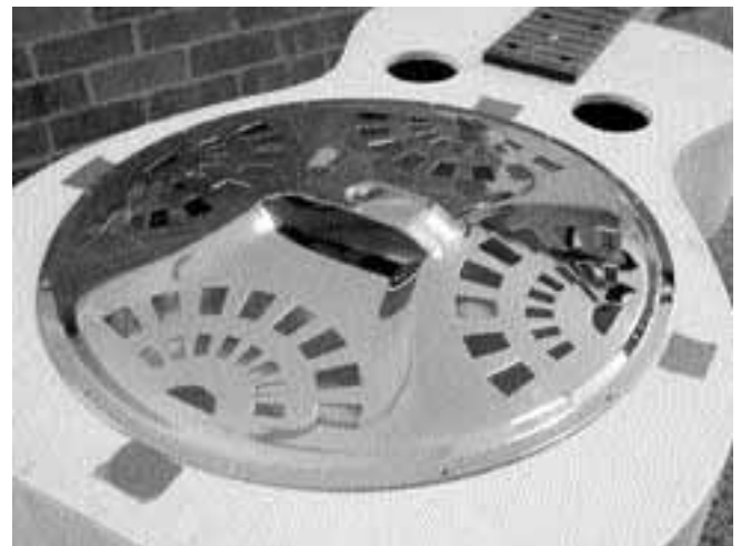
54. The cover plate should center between the markers.
