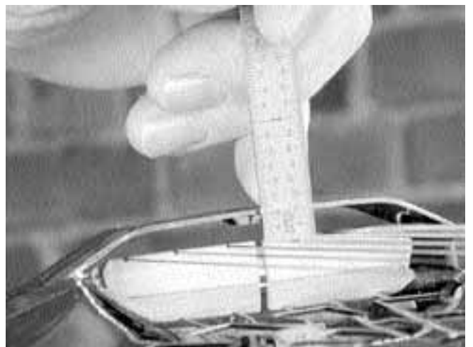
55. Under string tension, our Blues Resomaster showed a clearance of 1/4" from the top of the strings to the underside of the hand rest.
