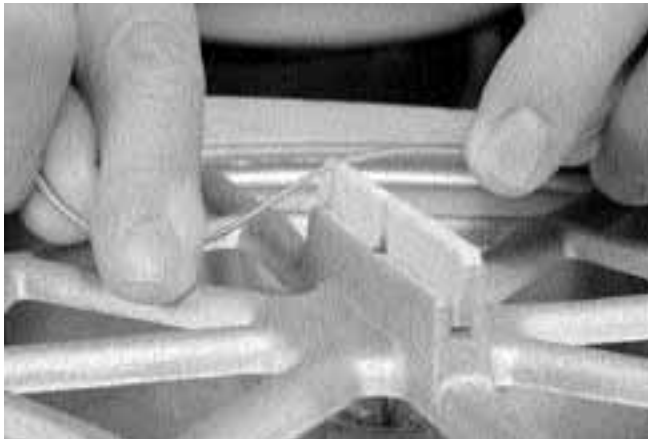
51. Burnish the saddle slots by working the strings back and forth through the slots.
