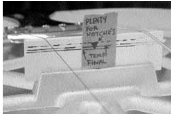
48. Approach the final action height slowly. Otherwise, you may waste a saddle blank.
