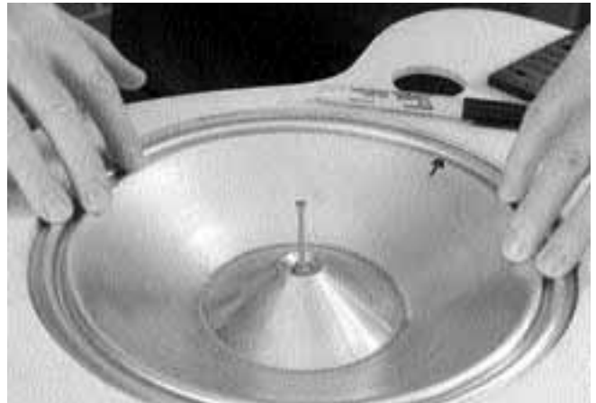
41. Set the cone on the rim. Rotate it until you find the cone's "sweet-spot." Mark the front of the cone with a felt marker.
