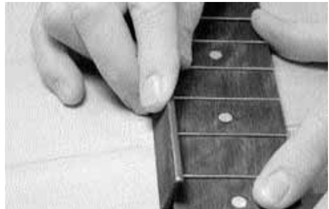
28. To bevel the fret ends, use a smooth mill file held at an angle.
