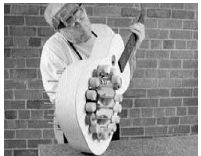
11. Apply Titebond glue, and clamp the sound well to the top with spool clamps.
