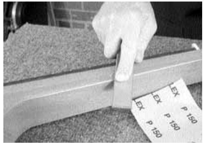
38. Use a file and sandpaper to round off the square machined edges of the neck and heel.
