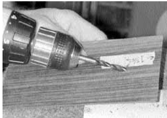
34. Hold the overlay in one hand and elongate the hole by slowly tilting the overlay against the running drill bit.
