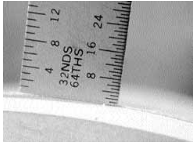
18. The router bit will cut slightly deeper than the actual thickness of the binding — perhaps by as much .007".
