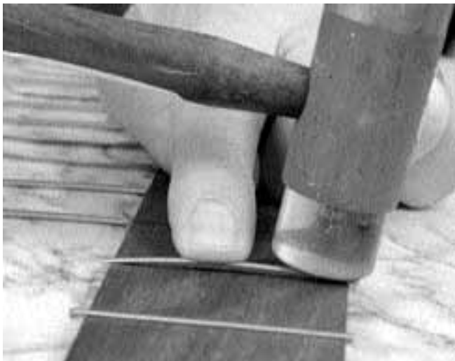
27. Keep the wire from tipping and prying up wood as you tap the two ends into the fret slot with a hammer.
