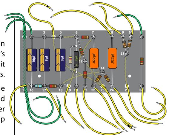
Now all the components and wires are on the eyelet board. Take a break to rest your eyes before making sure you've followed each step correctly. To find no mistakes at this stage is surprising, and it's much less work to find them now than after soldering!
