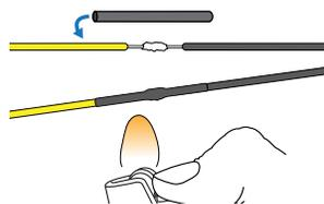
Once the heat shrink cools, twist these leads back up and tuck them in between the left side of the power transformer and the chassis wall.
