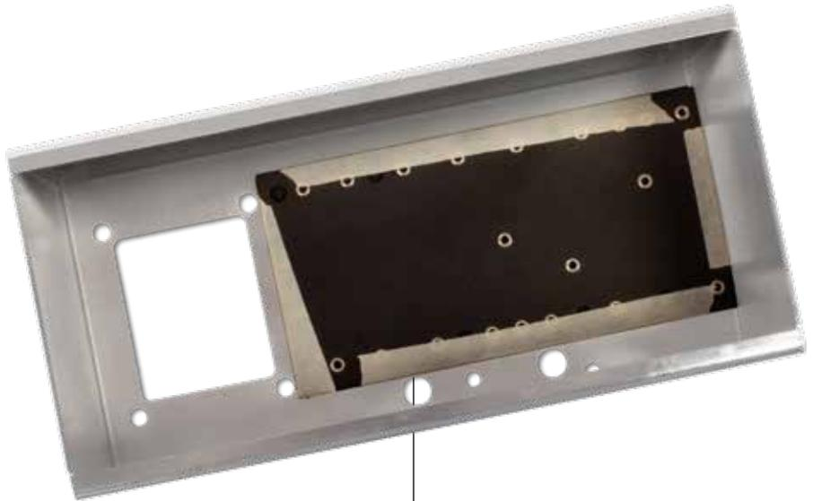
Position the taped boards inside the chassis as shown above, with a gap of roughly 1/4" between the boards and the top of the chassis. The ends of the boards are flush against the side of the chassis.
