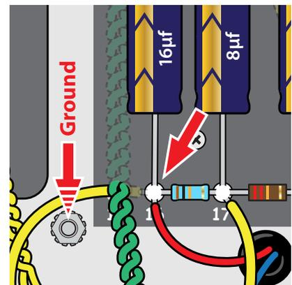
Set your multimeter to 500V DC and connect the black (negative) probe to ground. Once that probe is secured to ground, measure the DC voltage at eyelet 16. This B+ voltage should be roughly 479V DC.
