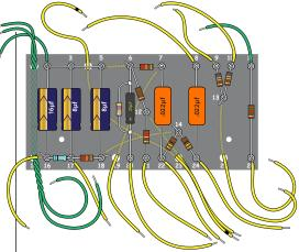
Now all the components and wires are on the eyelet board. Take a break to rest your eyes before making sure you've followed each step correctly. To find no mistakes at this stage is surprising, and it's much less work to find them now than after soldering!
