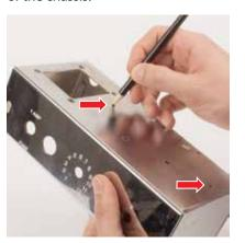
Holding the boards in place, turn the chassis so you can see the two mounting holes. Using a sharp pencil through the holes, mark the hole locations onto the insulator board. Drill the 5/32" mounting holes through the pair of boards. Separate the boards and set the insulator aside for later.
