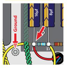
Set your multimeter to 500V DC and connect the black (negative) probe to ground. Once that probe is secured to ground, measure the DC voltage at eyelet 16. This B+ voltage should be roughly 479V DC.
