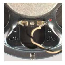
Before soldering these leads, place a business card or other protection under the terminals to prevent solder dripping onto the speaker cone. Solder the two leads to the speaker terminals. See "Tips for great soldering" on page 16.
