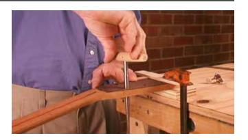
Holes for non-tapered press-in bushings may require a countersunk hole, or careful filing to enlarge the reamed tapered hole. After you have fit the first bushing, use the peghole as a reference and wrap tape around the reamer as a depth stop for the remaining holes.
