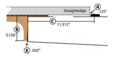
The measurement we want is **X** — the amount of wood to remove from the heel to change the neck angle so that a straightedge laid on the frets will be flush with the top of the bridge.
