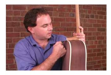
to side. If you need to remove a lot of wood, make two or three passes before changing to the other cheek. The fit will change rapidly, so check your progress frequently. A small ledge of unsanded wood will remain on the bottom of the heel between the sanded cheeks. Either "pull-sand" it with the strip, or use a sharp chisel to remove it.
