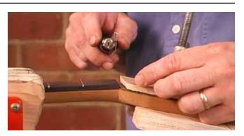
Lightly glue the nut in place with a couple of drops of Titebond in the mahogany slot, and a couple of drops on the end of the fretboard. You can sand the edges of the nut when you final-sand the neck.
