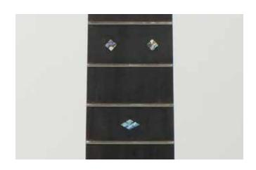
Use just a touch of super glue or black epoxy to permanently set your inlays. The inlays are a tight fit, so you may need to press them flush to the surface of the fretboard using a hard, flat object. Use wax paper placed between the them—you don't want to have the object glued to your fingerboard if there is any glue squeeze-out. After you press the inlays flush in the center of the fretboard, they will be raised slightly at the edges, since the fretboard is radiused. Use a smooth
