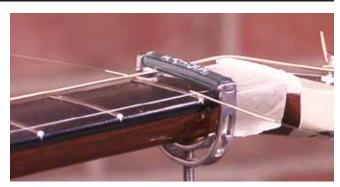
bottom of the strings and the top of the first fret. Set this clearance at about .020" below the treble E-string, and .030" below the bass E-string. Use .020" and .030" guitar strings to measure the clearance as the capo is tightened (pictured). Now measure the overall string action at the 12th fret. A
