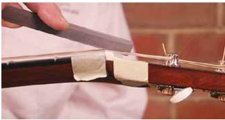
it upward gently. Place the nut in a vise, and file down the top surface until the slots are approximately half as deep as their string diameters. Re-contour the upper edges of the nut, using a file, sandpapers and polishing compound.
