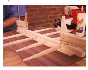
the distance of the spruce center strips. This keeps the reinforcing center strips in a neat, straight line from end to end. Use scrap wood cauls and two cam clamps for uniform pressure on each spruce strip. Avoid glue squeeze-out that might stick to the notched caul!
