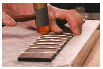
the fretboard extension over the body, will be installed later, after the neck is "dry-fitted" to the body. We do this because the fretboard extension will curve slightly from fret compression, making sighting and fitting the neck more difficult.
