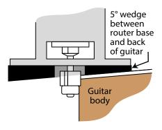
Double stick tape the 5° wedge to the bottom of your router base. You'll use this wedge for routing from the neck block area all the way to the last brace in the lower bout. Once you get to the last brace, remove the wedge, read just the height of the bit, and finish the cut to the center of the tailblock before stopping again. This will be repeated on the opposite side of the body.
