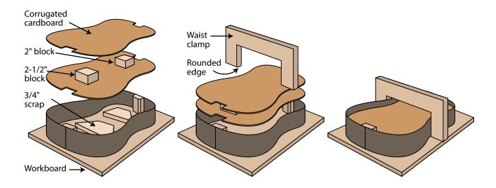
Next, glue a 2" thick block of scrap wood onto the cardboard, centered about 4" from the smaller end of the guitar mold. Then glue a second 2-1/2" piece of scrap wood, centered about 4" from the bottom (larger end) of the guitar mold. Glue the second piece of cardboard onto them. Now the two cardboard forms are fastened together with blocks of wood between them, creating a three-dimensional form for supporting the guitar sides.
