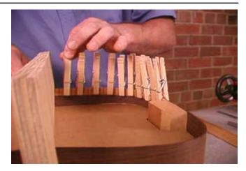
Titebond, check the 1/32" clearance and reclamp. Let the glue dry for 4 hours. Install the lining strips on the back edge of the side assembly in the same manner.
