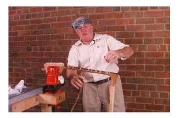
the neck. Tie the rubber band at the nut end, and start wrapping (**pictured**). The fretboard will align itself as you wrap, and can be easily moved if one edge is off-center. Stretch the rubber band tightly as you wrap toward the neck heel, go around the neck joint and the heel, and then wrap back to the nut. Even with a light glue application, you'll probably get a lot of glue squeeze-out. Wipe off excess glue and let the neck dry overnight.
