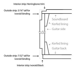
The first pass is for the interior strips and is made with the appropriate bearing on the cutter bit. The router bit should be set to cut a shallow ledge and a width to accommodate both the interior strip and the outside ivoroid binding. Make practice cuts on scrap wood, check the fit of the trim strips before routing the actual channels. Once starting the routing on the guitar body, check the fit before going very far to be sure both the depth and the width are correct.
