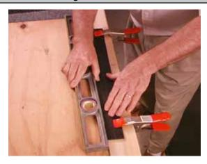
A shooting block is a long, square-edged sanding block for creating smooth, straight surfaces. We used a carpenter's level and fastened the sandpaper to it with double-stick tape (pictured).
