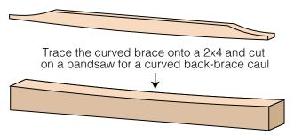
After applying glue to a brace, place the caul on the outer side and clamp the caul and the brace ends first (spring clamps are useful for this). Add two cam clamps to reach the center of the brace.
