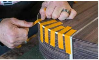
Binding the back: glue the thin ivoroid/black purfling first (ivoroid side in, black faces out) followed by the thick ivoroid binding. The binding joints at the neck block and tailblock must be trimmed for a close fit (**pictured**). Bind-ALL is a solvent based glue, so it will melt the joints together. Allow 6-8 hours drying time before removing the tape.
