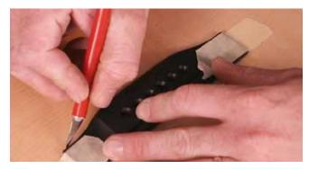
center and sides of the bridge (**pictured**). Use a hand plane, file or sandpaper to match the bridge's contours, and glue sandpaper to the bottom of each caul to help keep it steady when clamped.
