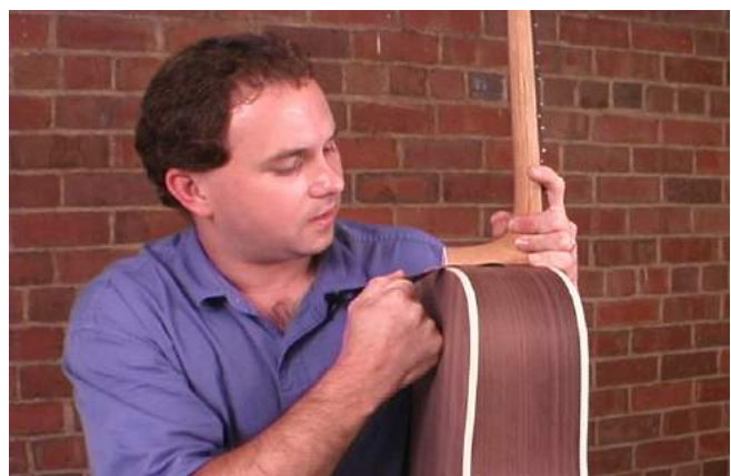
Removing wood at the bottom edge tips the neck back
