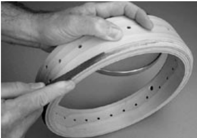
If necessary, file a small amount of wood from the tapered sidewall.
