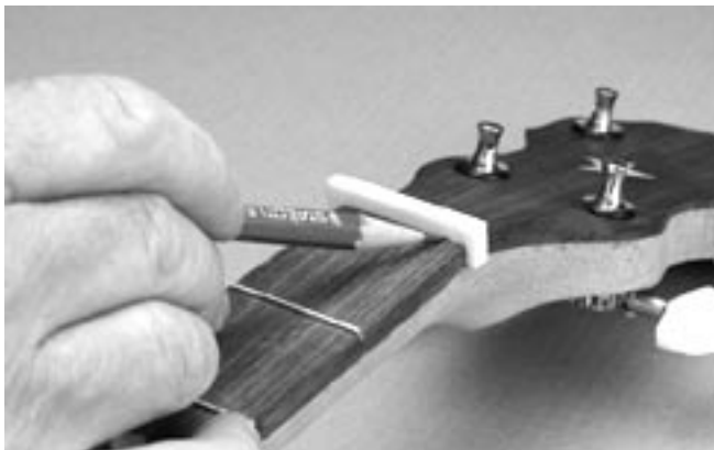
Draw a line across the fretboard surface onto the nut.
