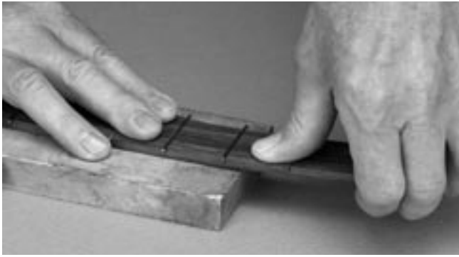
"Massage" out a backbow. Squeeze, don't force!
