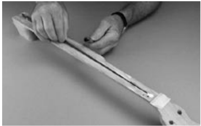
Use a thin, uniform coat of glue for the fretboard.
