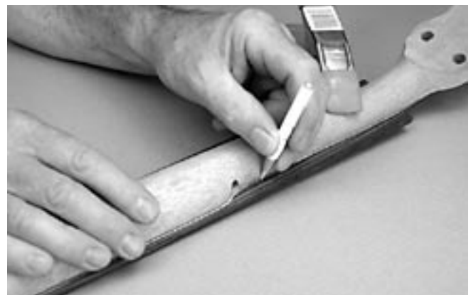
Pencil the neck's shape onto the fretboard.
