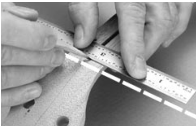
Pencil a line \frac{3}{16} " back from the break angle (dotted line).
