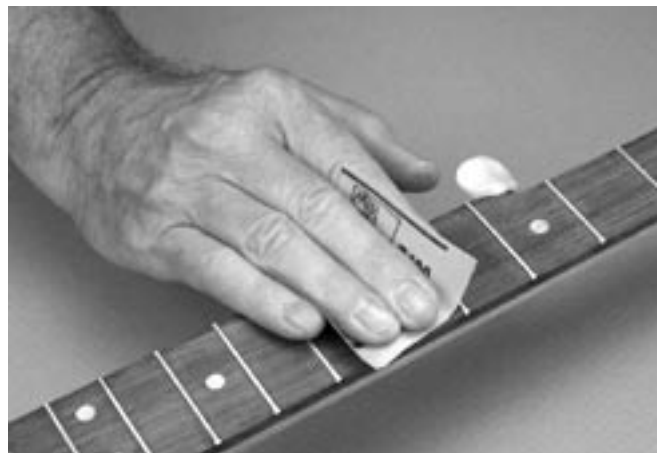
Wrap two fingers with sandpaper, and sand over the fret tops from end to end.
