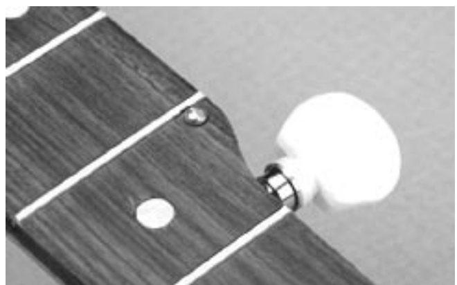
Align the screw slot to guide the fifth string up and over the fret.
