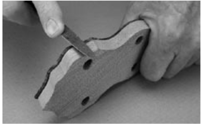
Carefully trim the peghead overlay flush to the peghead.
