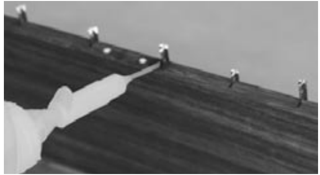
Run superglue into the ends of the fret slots.
