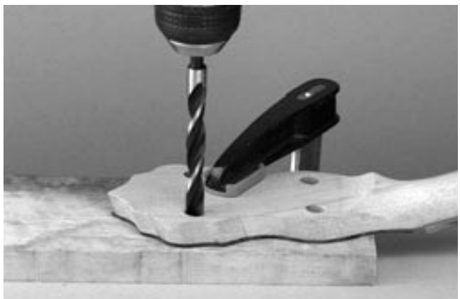
Drill through the overlay with a 3/8" brad-point bit.
