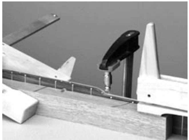
A good clamping setup for installing a 5th string peg. Press the 5th string peg into the hole slowly.
