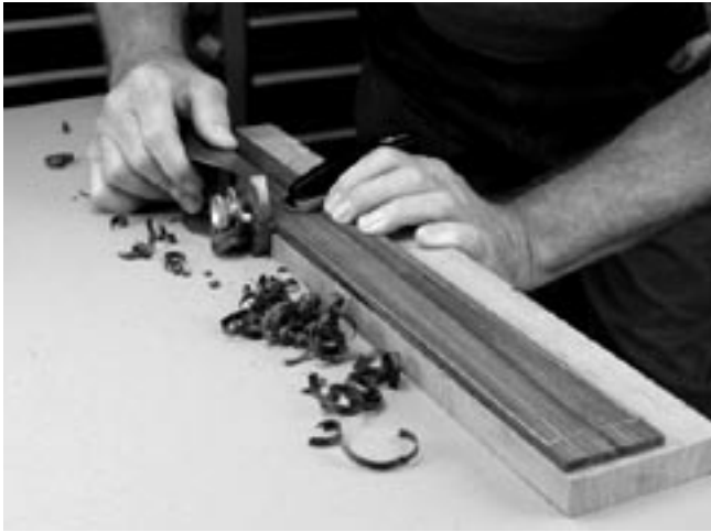
Using a block plane to trim the finger board.
