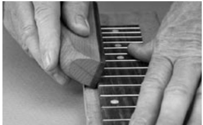
Bevel the fret ends.
