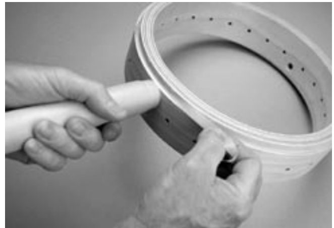
Use a length of wood dowel as a handle during finishing.
