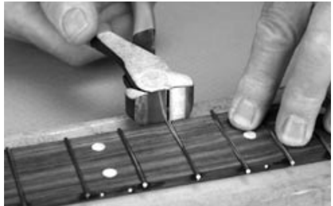
Nip the overhanging fret ends.
