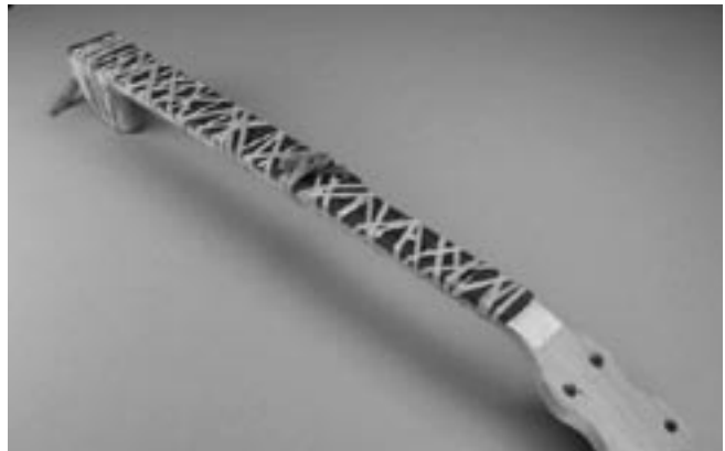
Align the fretboard on the penciled nut line, and wrap with the rubber band.
