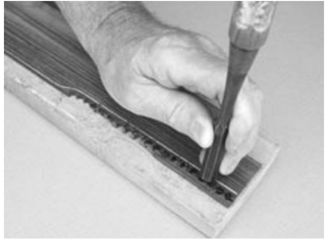
Drill a series of 1/4" holes, then chisel and file to shape.
