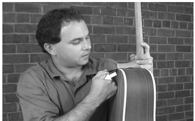
Removing wood at the bottom edge tips the neck back
