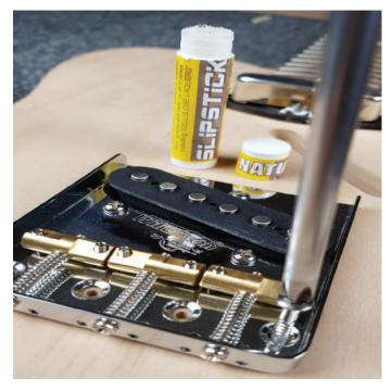
Drill the 4 bridge mounting holes deeper to accomodate the screws using a 1/8" drill. Mark the depth of the screw with tape on the drill after comparing the screw length. Countersink the hole slightly to avoid tearout when fitting the screws. Mount the pickup in the bridge and attach the assembly to the guitar. Lubricatring the screw with a small amount of Slipstick will make the assembly easier
