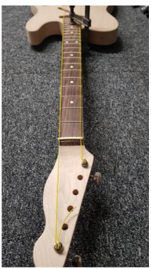
To align the neck and body I like to use a length of string/twine or thin hook up wire threaded through the E string ferrule holes in the body and then run the wire/ string up the neck through the nut to the E tuners to check alignment and make side-to-side adjustments to the neck as needed to make sure the strings ride even along both edges of the fretboard.
