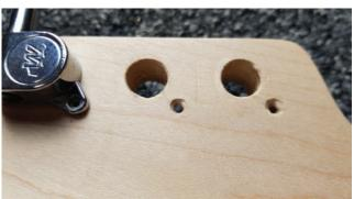
Lubricate the screw threads with the Wilkinson Slipstick provided in the kit. With the tuners in place, install the screws in the pilot holes with a #1 Phillips. Whenever you drill a hole be sure to countersink slightly larger than the screw diameter. this will reduce wood tearout and make for a clean assembly.
