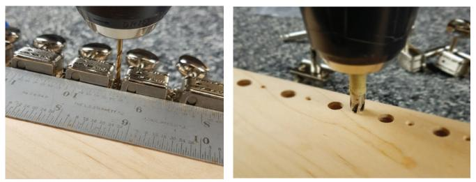
Mark out your mounting holes with a scribe or punch. Tuner mounting screws are very delicate and will break off if forced into hard maple. Use a 5/64" drill bit to make pilot holes for the screws; if these holes are any smaller you risk shearing off the screw heads.
