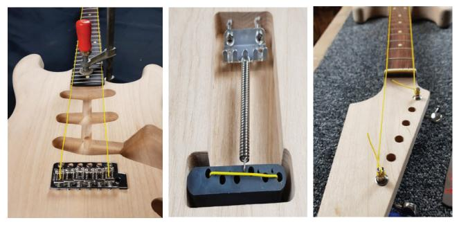
To align the neck and body I like to use a length of string/twine or thin hook up wire threaded through the E string holes in the block and then run the wire/ string up the neck through the nut to the E tuners to check alignment and make side-to-side adjustments to the neck as needed to make sure the strings ride even along both edges of the fretboard.
