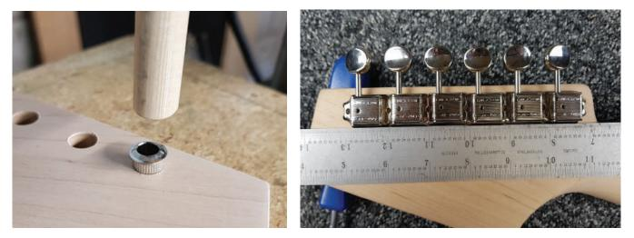
Lay out the tuners using a ruler to make sure they're in line with one another and square to the edge of the peghead.
