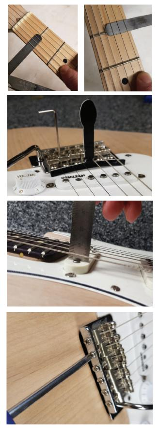
Sight down the neck and check for any Over bow (bending backwards causing string buzz on an open string or Under bow on the neck causing a higher than necessary action in the midle of the neck when playing. Adjust the optimum action with the truss rod.
